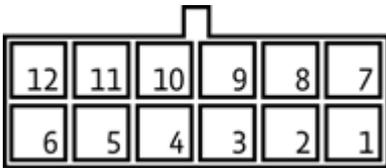
Figure 1: I/O Connections (top view)
