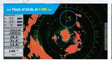
At 4 NM the bird echoes are extremely clear, and distinctly visible compared with other targets.
